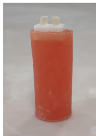
Figure 1: Zirconia cube mounted in an acrylic block with 4 cylinders made with resin cement
