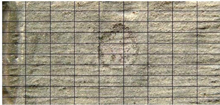
Figure 5. Broken specimen with soldering at x10.5 magnification
