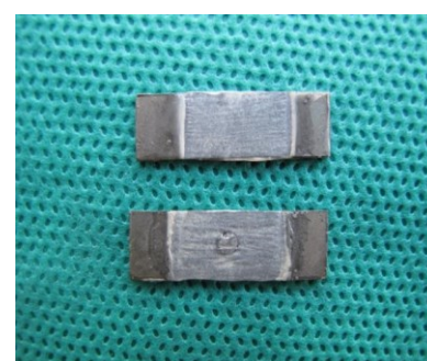
Figure 3. Broken specimens with/without soldering
