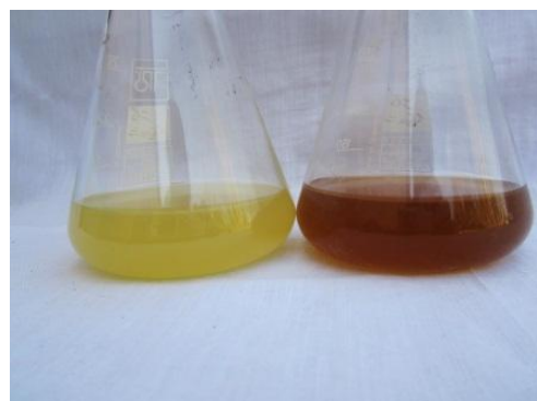
Figure 1. Biosynthesized gold nanoparticles in a colloidal dispersion by Streptomyces fulvissimus isolate U colonies before (left) and after (right) exposure to HAuCl 4 after 48 h.
