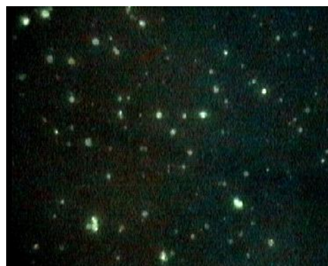
Fig.1. Fluorescent microscopic image of particles coated with FITC-BSA, prepared by single emulsion method
