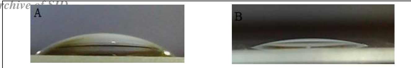
Fig. 4. A water droplet on A) the non-treated surface that produced 30° angle and B) 150 s helium-treated surface that produced a 10° angle
