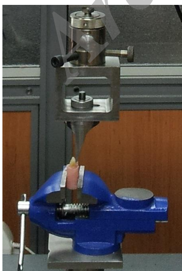
Figure 1: The specimen under the shear bond strength test using the Universal Testing Machine.
