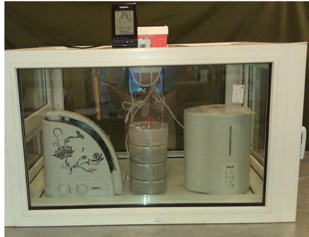
Figure 2: Humidity and temperature simulator for oral cavity which were especially designed for this study by Moazzami et al.
