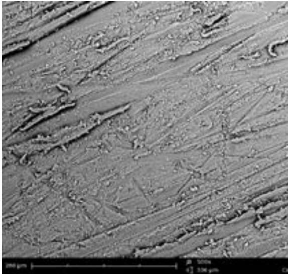
Figure 1-a: The surface roughness of a specimen in the control group at 500X
