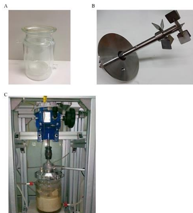
Figure 1. The vessel, mixing system and bioreactor. A) The vessel was built using Pyrex and equipped with an external jacket that allowed the circulation of service fluid necessary to maintain the entire apparatus at a constant temperature. B) The stainless steel impeller with two various types of turbines: a blade turbine to reach an axial flow and a Rushton turbine to reach a radial flow. C) The complete equipment was used for the lab-scale experiments.
