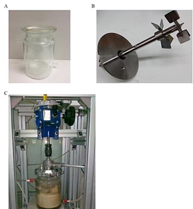
Figure 1. The vessel and the mixing system. A) The vessel was made of Pyrex glass. It included a jacket vessel; in which, the thermo-stated water was circulated; B) The stainless steel impeller with two various types of turbines: a blade turbine to achieve axial flow and a Rushton turbine to achieve radial flow; and C) The complete equipment used for the laboratory-scale experiments.
