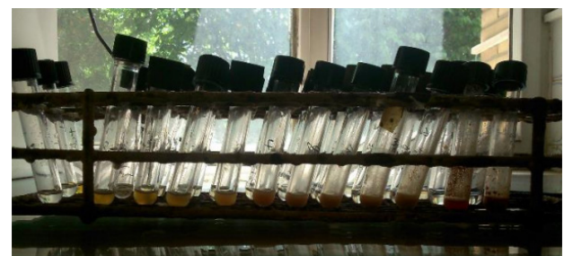
Figure 1. Different Concentrations of GSE Added with 0.5 mL of Prepared Microbial Suspensions. Note. GSE: Grape seed extract.
