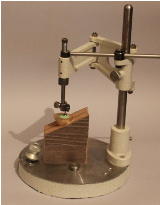
Figure 3. Analog Positioning in Brass Mold Using a Surveyor.
