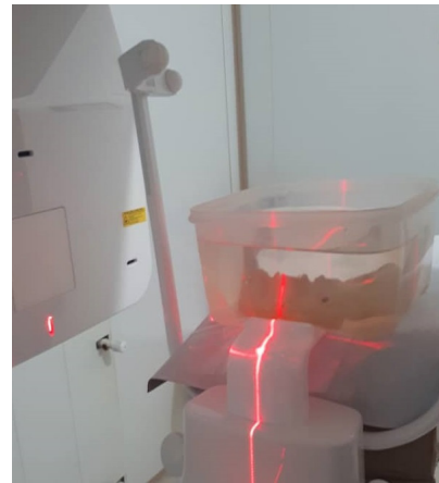
Figure 1. Dry Mandible in Water Box Mounted for CBCT Imaging.
