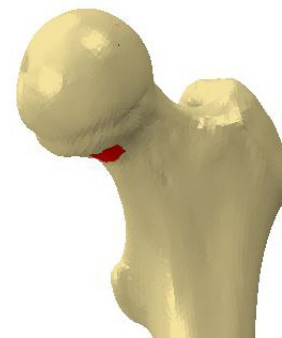
Figure 3. The most probable region of femur fracture subjected to the loadings used in the reference model with normal bone density. The stress in the red region exceeded the Mises criterion limit of failure.
