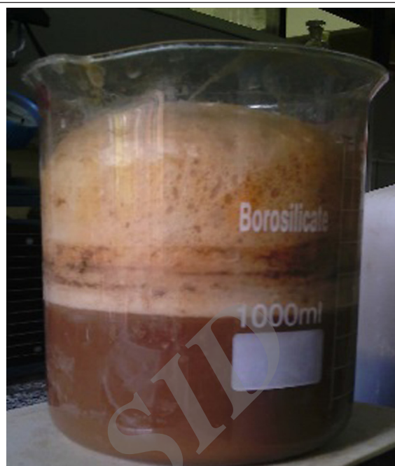
Figure 2. The Formation of Foam Due to the Presence of CO 2
