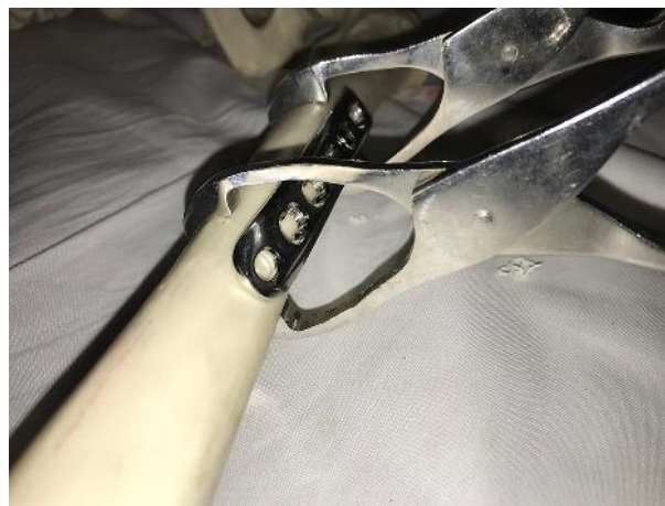
Figure 3. Experimental assessment of plate insertion by the new designed device
