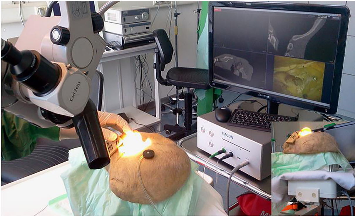
Figure 1. System setup, a hardware module, application software, the magnetic field, generator and specific sensors that fix the head
