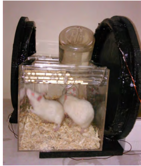
Figure 1. Animals placed in the Plexiglas exposure Cage within the Helmholtz coils
