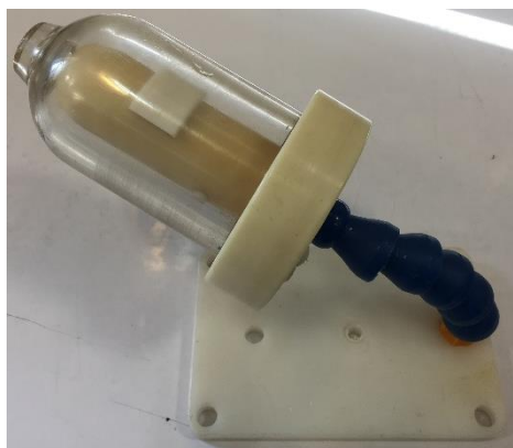
Figure 2. An in-house heart phantom to assessing image quality of the ProSPECT system
