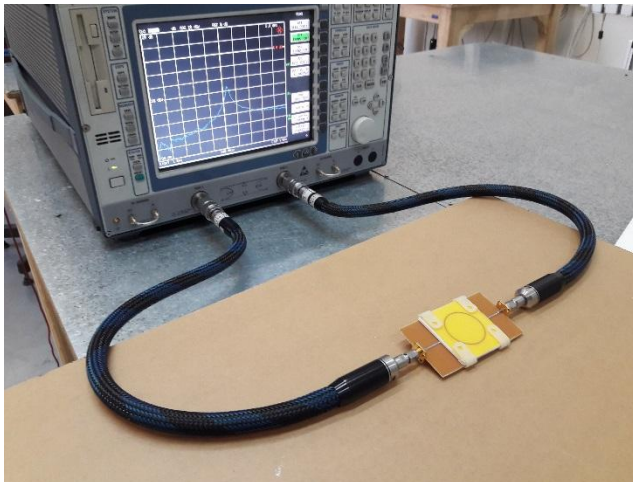
Fig. 9. Measurement setup for the fabricated circuit.
