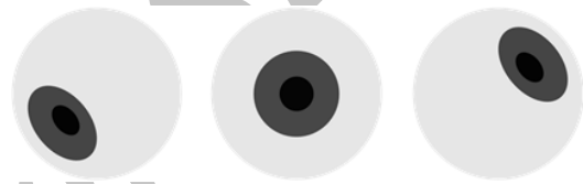
Fig. 5: Three different gaze directions and their effects on the 2D images of the iris boundary and the pupil position.
