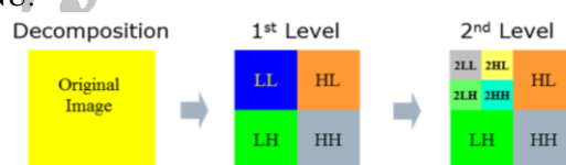
Figure 2: Bands of wavelet transform to the level 2
