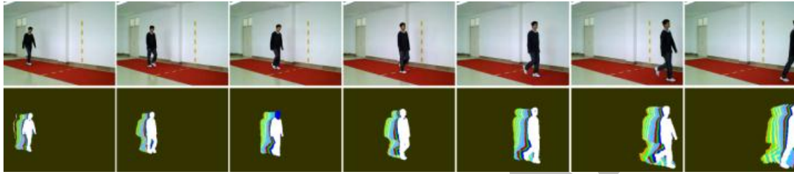
Fig. 4. Motion History Images (left to right and bottom column) for 95 to 170 frames, 95 to 110 frames, 105 to 120, 115-130, 125-140, 135-150, 145-160, 155-170 frames of a sample video sequence or 132 video frames.
