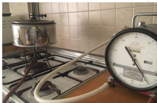
Figure 2. The experimental equipment including gasometer, Bunsen burner, and double wall container
