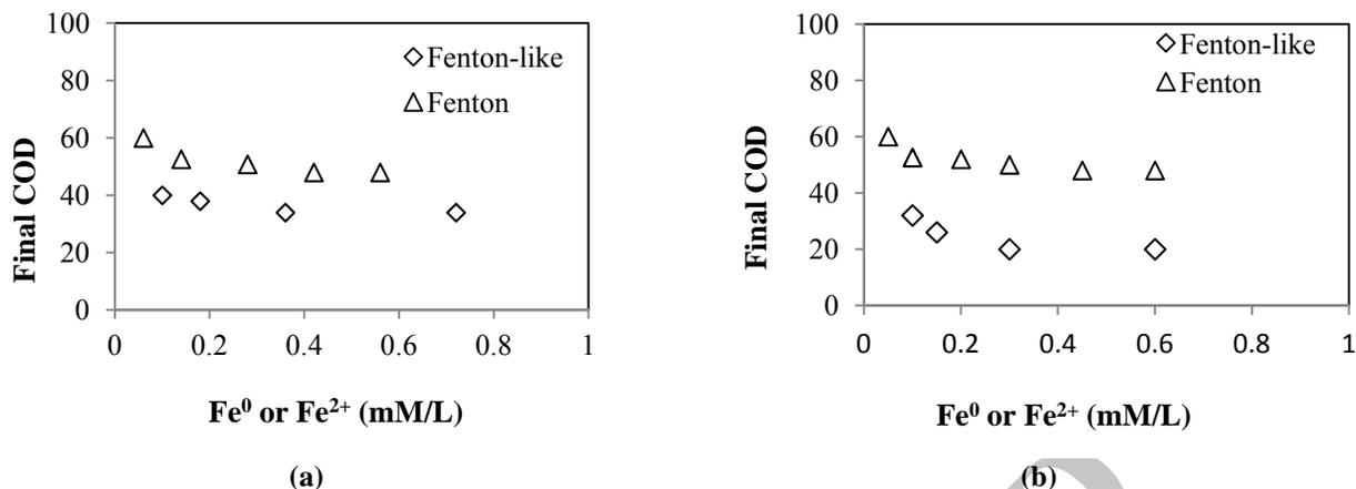
Figure 4) Effects of Fe<sup>0</sup> or Fe<sup>2+</sup> on chemical oxygen demand (COD) removal rates obtained for azithromycin (a) and clarithromycin (b) antibiotics by “Fenton” and “Fenton-like processes”
