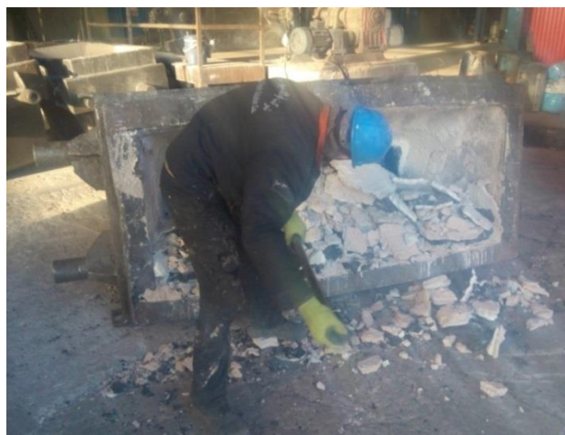
Figure 1) The posture destroying the Tundish work before the correction
