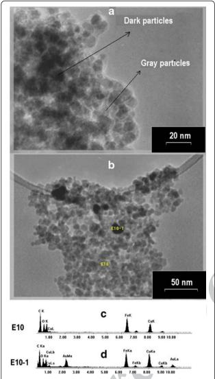
**Figure 2 Transmission electron microscopic images.** Of both magnetic-gold composite nanoparticles (dark particles) and bare  $Fe_3O_4$ magnetite nanoparticles (gray particles), recorded by different magnification (**a** and **b**). Lower illustrations show energy-dispersive spectroscopy patterns of these gray (**c**) or black (**d**) nanoparticles.
