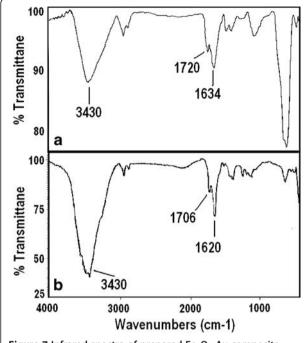
**Figure 7 Infrared spectra of prepared Fe<sub>3</sub>O<sub>4</sub>-Au composite nanoparticles.** Before (**a**) and after (**b**) acid wash treatment by HCL (1 N).
