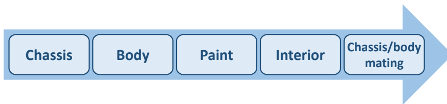
Fig. 5. Major Processes of a Car Assembly Line
