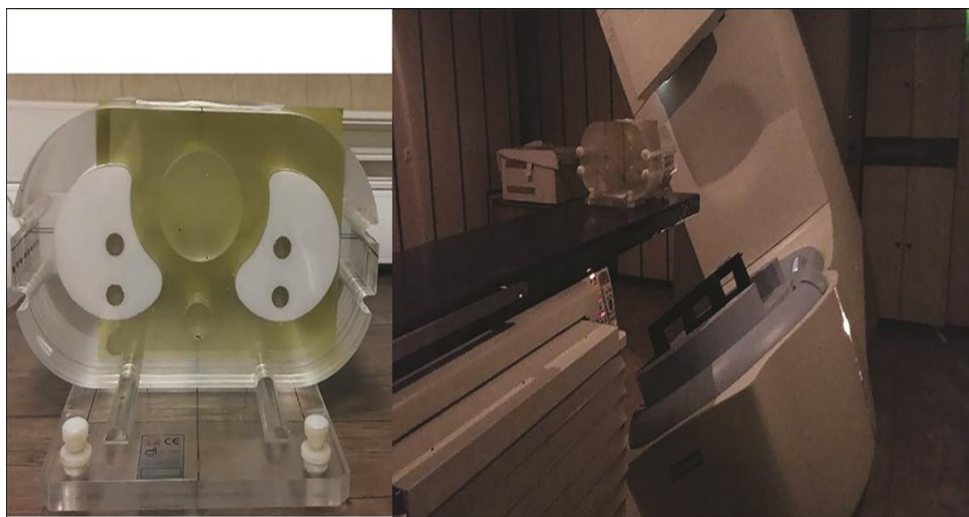
Figure 3: EBT3 film sandwiched between the inhomogeneity phantom for IMRT QA and irradiated with 6MV ONCOR linear accelerator.
