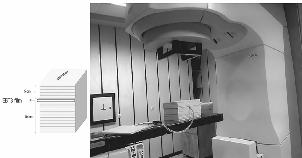
Figure 2: Solid water phantoms and EBT3 film that was sandwiched between them in order to obtain calibration curve.
