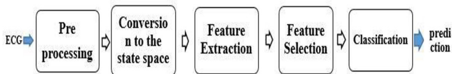
Figure 2: The block diagram representing the proposed algorithm.
