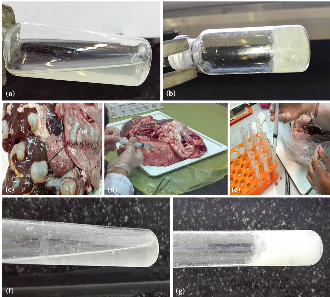
Fig. 10 a Polymer solution at 4 °C with CS/CMC ratio of 1.75/1.4 and BGP (2.9%), b formed gel at 37 °C, c contaminated liver hydatid cyst, d aspirated HCF, e sterilized HCF, f injected polymer solution
