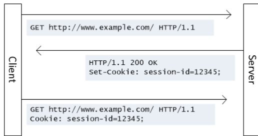
Figure 2. The request process in the HTTP protocol
