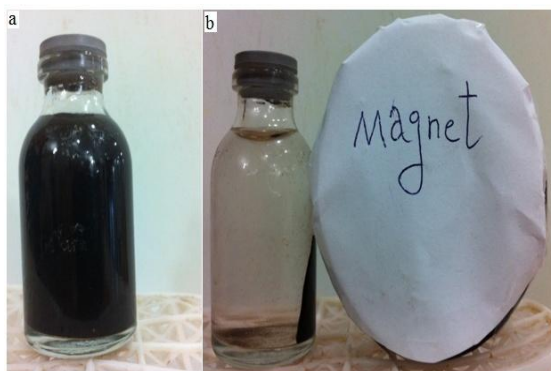
Scheme 2. Nanomagnetic acid catalyst: a) disperse b) separated by an external magnet
