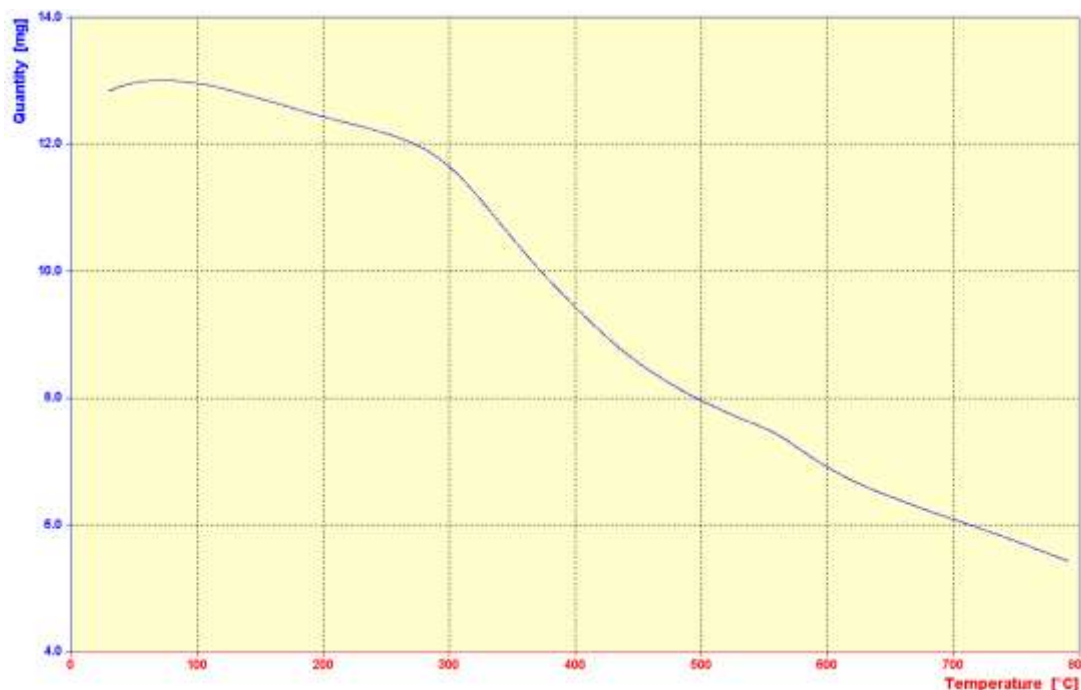
Fig. 6. TGA curve of superparamagnetic carbonaceous material functionalized with sulfonic acid groups ( \text{Fe}_3\text{O}_4@\text{C}-\text{SO}_3\text{H} ).
