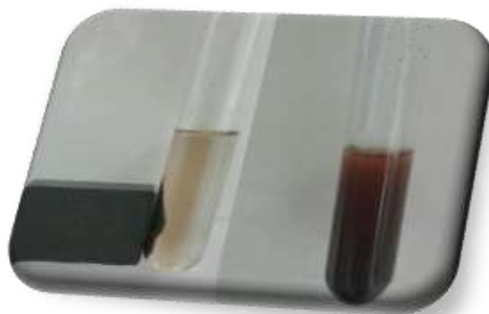
Fig. 1 The separation of catalyst by an external magnet
