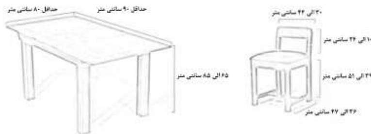
Figure 2. Ergonomic dimensions of suitable furniture for making jewelry
