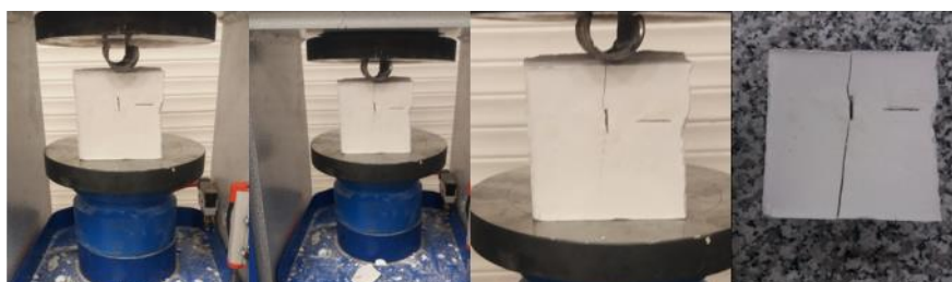
Figure 3. Failure pattern of non-persistent joint
