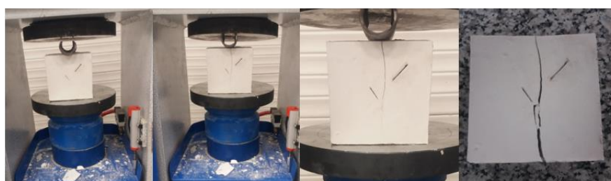
Figure 4. Failure pattern of non-persistent joint
