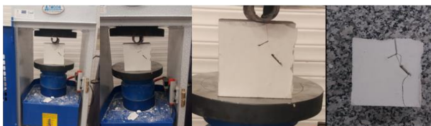
Figure 2. Failure pattern of non-persistent joint
