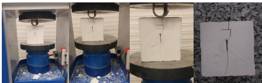
Figure 1. Failure pattern of non-persistent joint
