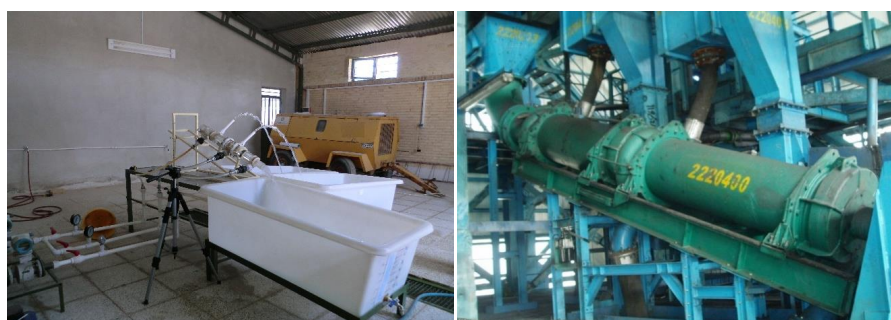
Figure 1. Tri-Flo separators used in this study (left: laboratory, right: industry)
