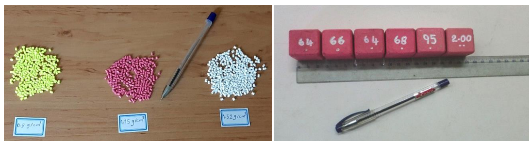
Figure 2. Density tracers used in this study (left: laboratory, right: industry)
