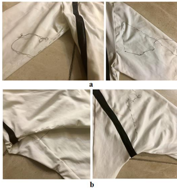
Figure 6. Metal yarn in the proposed full body swimsuits with (a) drop sleeves and (b) raglan sleeves.
