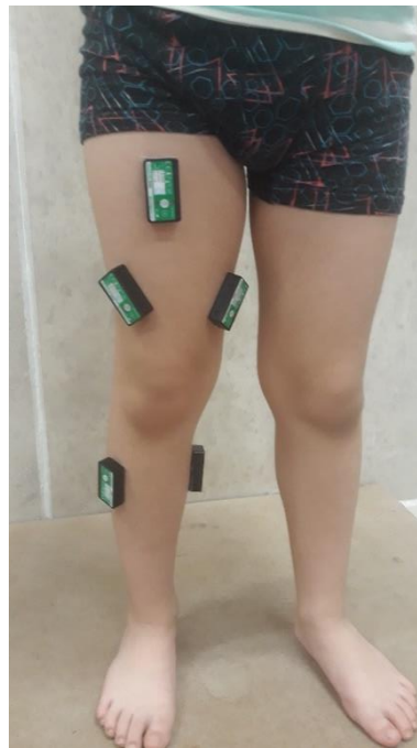
Figure 1: Electrodes positions in according to SENIAM recommendation
