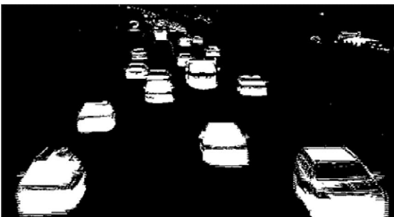
Fig. 9. A differential image using Imfill operator
