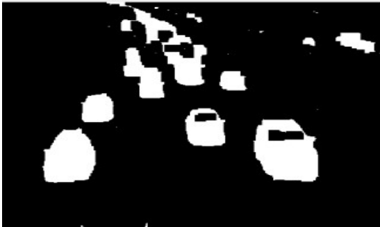
Fig.8. A differential image using close operator
