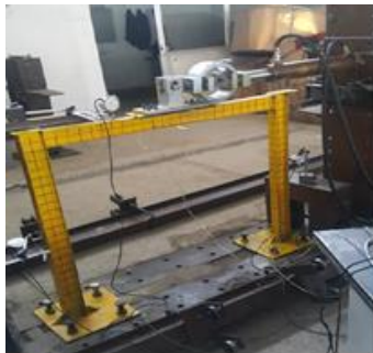
Fig. 2. Experimental specimen of N1 steel moment resisting frame
