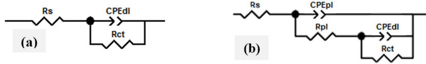
Fig. 6- The equivalent circuits used to simulate corrosion behavior of samples in a) inhibitor free and b) SP-containing artificial sea water using EIS measurement.
