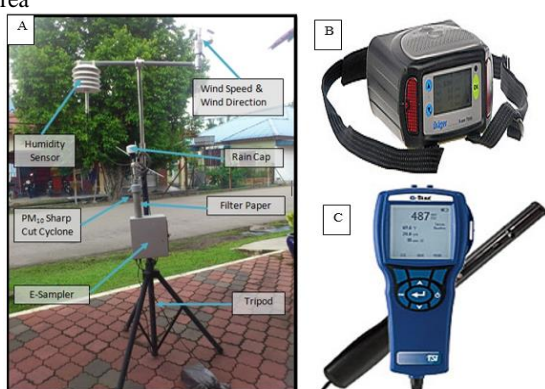
Figure 2 Sampling instrument; 1) E-sampler Particulate Matter used for PM 10 determination and meteorological parameters, 2) Dragger X am 7000 Used for determination CO concentrations; 3) TSI IAQ Monitor Used for determination NO concentrations
