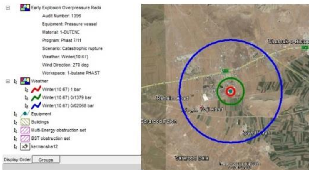
Fig. 1: The affected area by vapor cloud explosion due to full rupture of the reservoir in the winter.
