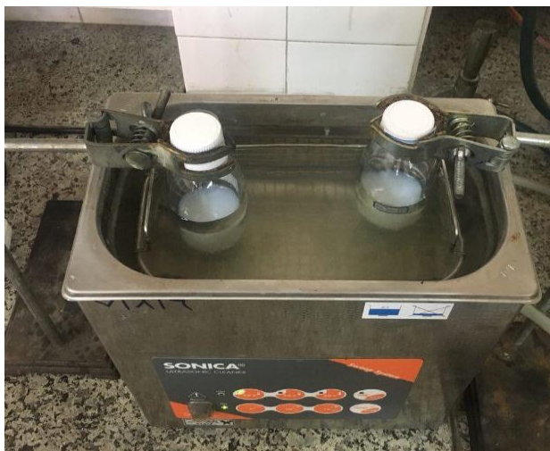
Figure 5- TiO 2 nanofluids under sonication by bath sonicator
