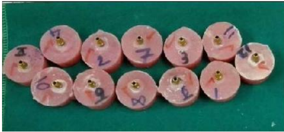
Figure 2. Implant-abutment assemblies mounted in a block of acrylic resin.
