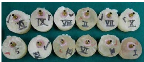
Figure 2. Case and control samples mounted in resin blocks
