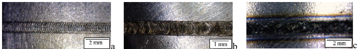
Figure 6. Surface appearance of A series: (a) A_1 (100% Ar), (b) A_4 (85% Ar + 15% \text{CO}_2 ), (c) A_6 (75% Ar + 25% \text{CO}_2 ).
