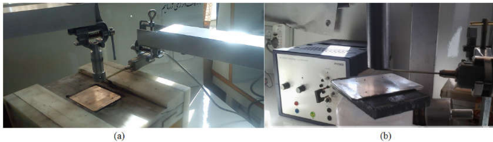
Figure 20. (color onlin) Magnetic flux density measurement. a) all parts are non-ferromagnetic, b) work piece fixture and magnet are ferromagnetic, while the work piece is non-ferromagnetic.
