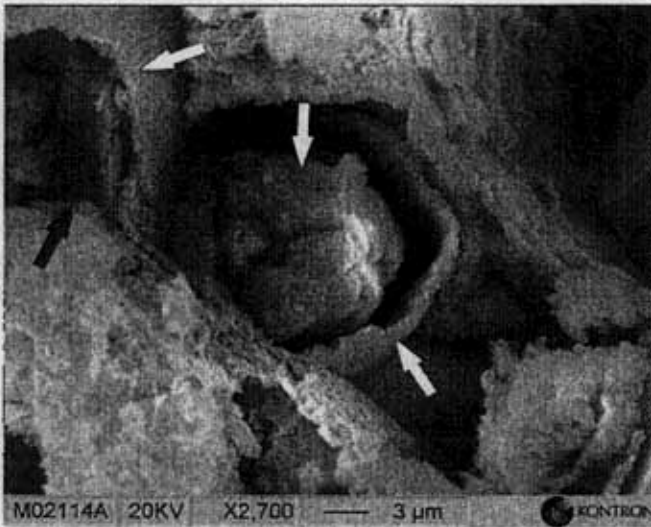
Fig. 3 SEM-photograph of a typical boxwork structure, which consists of 'onion-skins' of porous goethite (white arrows), containing some 15% Zn and relict core (black arrow) of partly dissolved hemimorphite (type-1).
